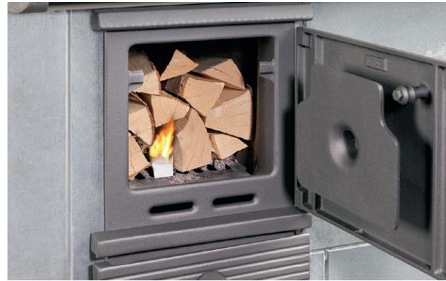
Set out 2 kg (4 lbs) of firewood that has been chopped into small pieces in a way that encourages air flow (approx. 10 pcs). Light the firewood from below using firestarter block and close the door. Adjust the service door a bit open using the door handle.
