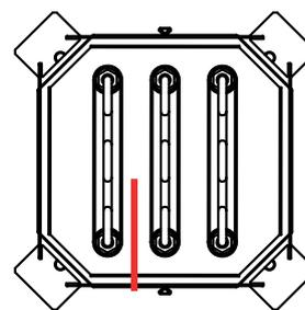
2. Pass the thermocouple through the hole near the top edge of the connection box.
