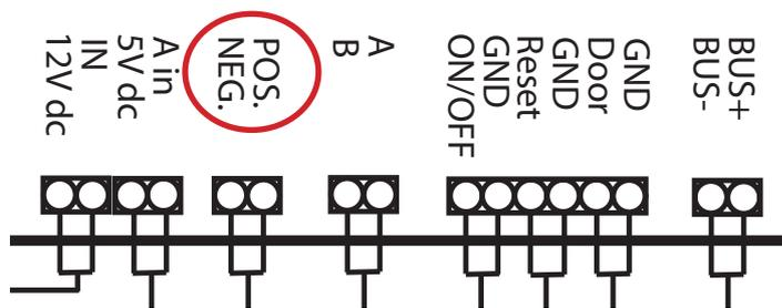
1. Connect the thermocouple to the sauna heater control card.
